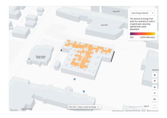
The map shows where the panels could be placed, and also has a feature that can generate the cost feasibility of each building as well. This is a more accurate way to measure the solar panel space than the team had previously considered.
